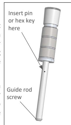
6. Replace one or more of the existing steel weights with the tungsten weights taking care to retain the placement of the rubber O-rings. One O-ring should be positioned on every side of the weights except in the space between the weight and the snap ring.
